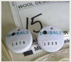
When collecting data in the project, the beacons will be inserted under the label on the wool pack (they are photographed here outside the label to demonstrate size). The beacon on the right is emitting a faint blue light from the middle of the beacon, indicating that the beacon has been connected to an iPad and is currently delivering live data. The beacon on the left is still collecting data, but not currently sending that data to a smart device.
